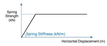
Spring Strength [kN] = Section Width [m]  $\times$  Element Length [m]  $\times$  PHU [kN/m<sup>2</sup>]
