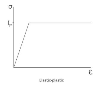
For some codes (CAN/CSA) the initial slope is reduced to  $\phi E$  .
