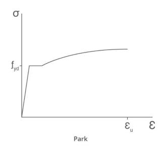
The steel stress-strain curve is characterised a liner response to yield, followed by a fully plastic zone, before hardening until failure.
