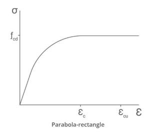
The parabolic curve can be characterised as
