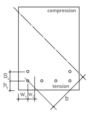
The first stage is to identify the most tensile bar and determine the cover c to this bar. We then define  $h_i$  as the cover plus half the bar diameter.
