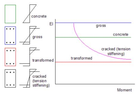
For a symmetric section, symmetrically loaded, stiffness can be expressed as
